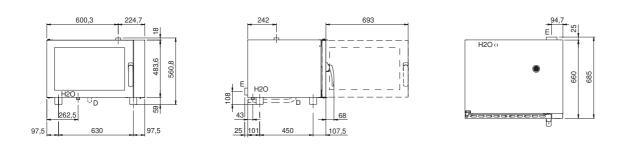
E: Electric connection D: Drain for water H2O: Water inlet 3/4"
