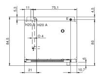
E: Electric connection D: Drain for water H2OA: Water inlet
