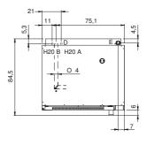
E: Electric connection D: Drain for water H2OA: Water inlet
