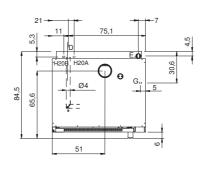
G: Gas connection E: Electric connection D: Drain for water
