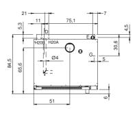
G: Gas connection E: Electric connection D: Drain for water
